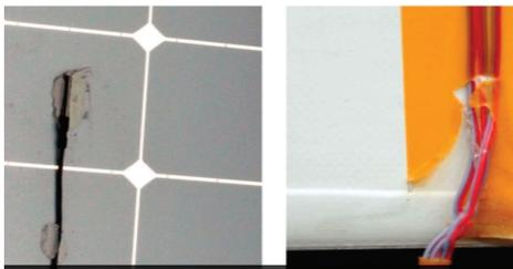
Fig.6. Temperature sensor attached on the PV panel
