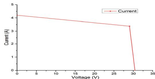
Fig.7. V-I characteristics at 28°C temperature level
