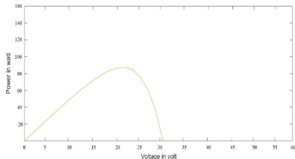
Fig.15. P-V characteristics of the solar panel at 28°C
