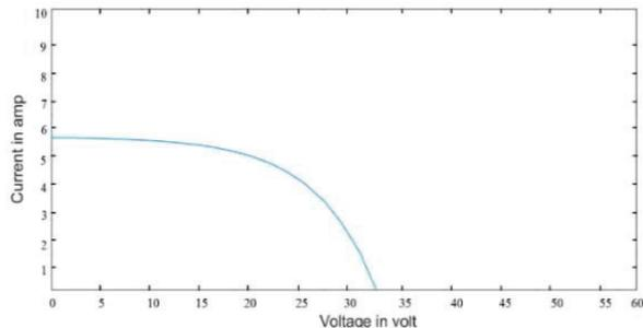
Fig.14. V-I characteristics of a solar panel at 28°C
