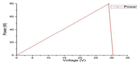
Fig.8. P-V characteristics at 28°C temperature level
