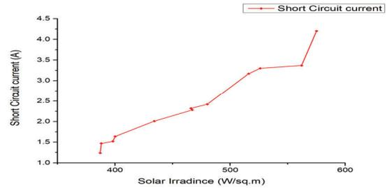
Fig.12. Irradiance dependence of Short circuit current
