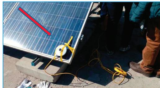
Fig.3. Pyranometer for irradiance measurement
