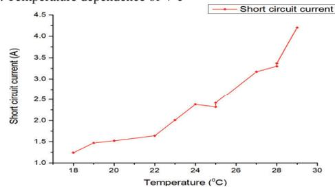
Fig.11. Temperature dependence of Short circuit current
