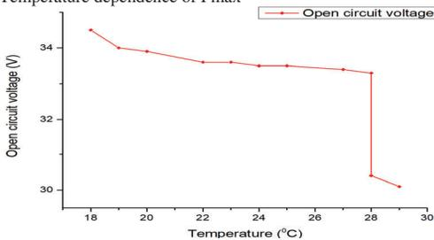
Fig.10. Temperature dependence of V<sup>o</sup>c
