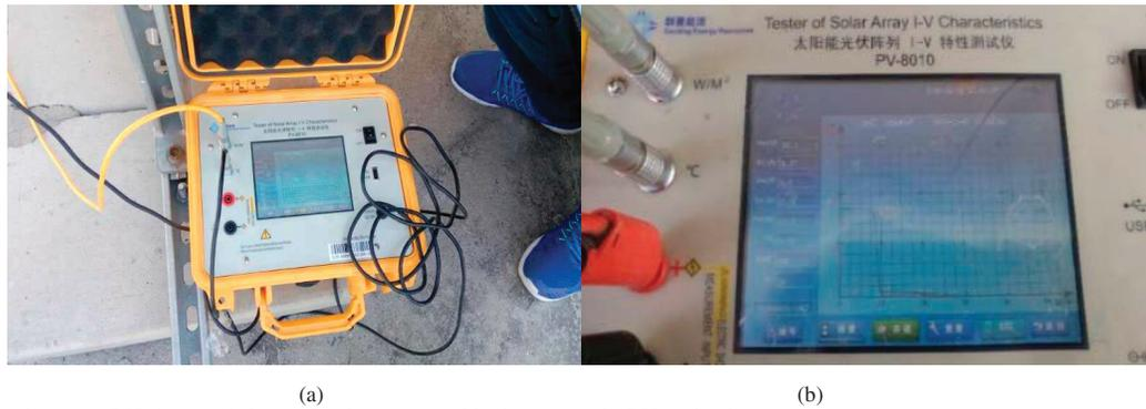
Fig.4. Tester of solar Array I-V characteristics (a) Device connected in the system (b) I-V testing in progress
