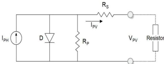
Fig.2. Electric circuit of a solar panel[15]
